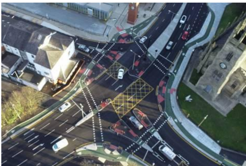
Example of a signalised junction with protected facilities for cyclists (Newport Street, Bolton)
